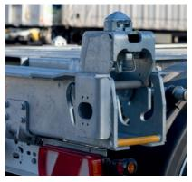
The height-adjustable **STEP LOCK®\*** on the rear extensionextension allows 40' and 45' containers to be40' and 45' containers without a tuppel
