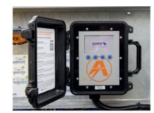
The **control panel** with TFT monitor displays operating status, consumption, total running time and the next maintenance date.
