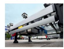
**130 litre diesel tank** for up to 60 hours of continuous operation of refrigerated containers. **High ground clearance** (approx. 310 mm).
