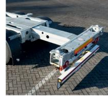
New: **Damped rear extension** moves **pneumatically** to the selected locking position and brakes gently.
