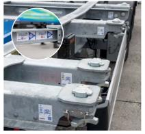
**New labelling** on locks and extensions for reliable identification of the different loading positions, supported by a loading plan and operating videos via QR code.
