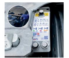
**Control unit for pneumatic locking** for the rear extension, optionally with manual lockingLocking\*.
