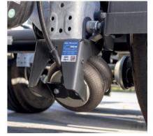
The **lift axle\*** as a starting aid extends the wheelbase and thus increases the pressure on the drive axle. Unloaded, the lifted position reduces tyre wear.
