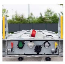
Recessed connection strip on the front beam with CEE socket\* on the beam for supplying refrigerated containers with Genset\*.
