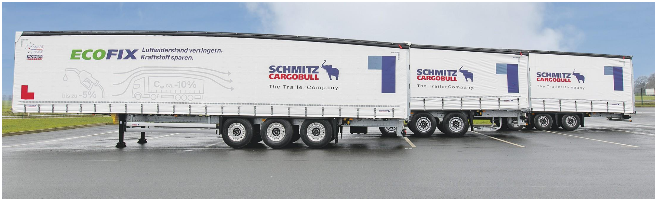
The rear shapes compared: On the EcoFIX with fixed aerodynamic geometry, the tarpaulin is super smooth. On the EcoFLEX (middle) and the EcoVARIOS high-volume model, the tarpaulin is not 100% smooth in the corner areas.
