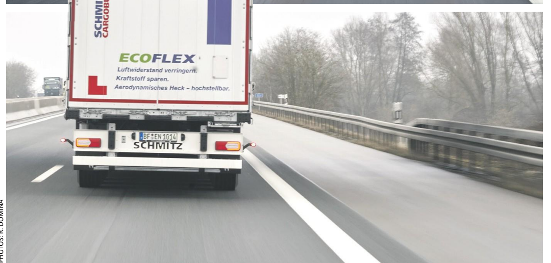
The lower rear section reduces the through-loading height of the rear doors by half a metre (from 2,550 mm to 2,050 mm).
