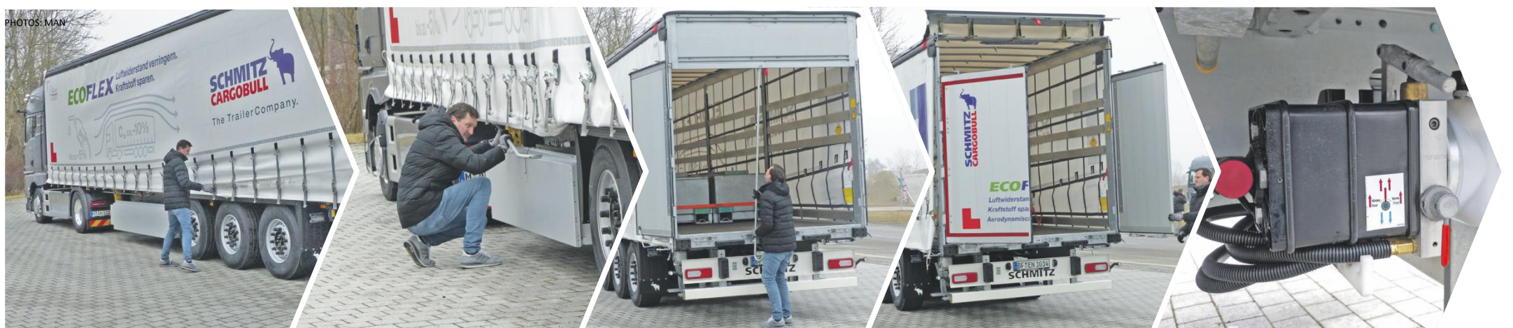
Converted in 20 minutes: It all begins with releasing the tensioning locks.
