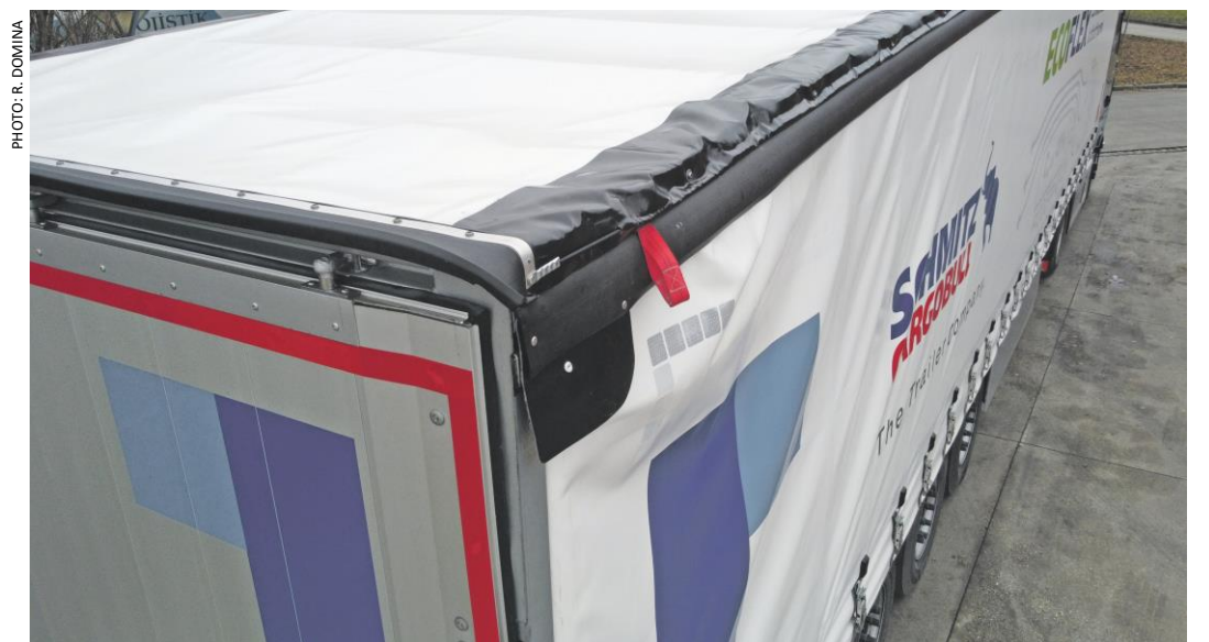
The curved side line changes the geometry of the side tarpaulin. The tie rod cannot roll up the excess, creating wrinkles. The developers are working on a solution.
