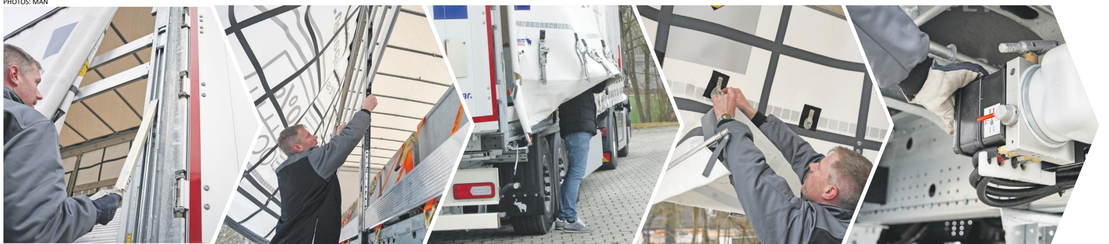
Now the height stops can be easily pushed into the aero position.
