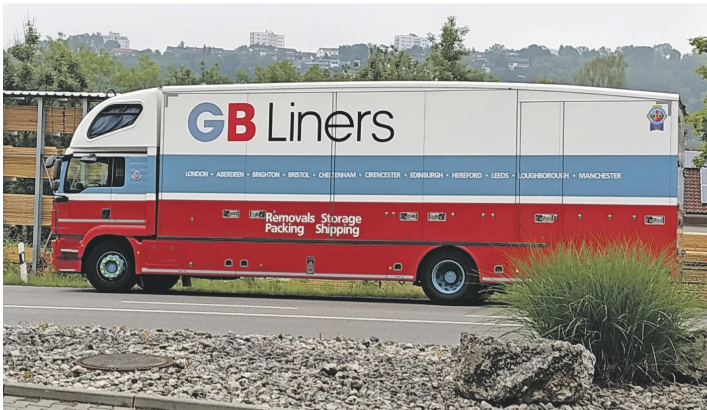
The shape of this British furniture truck exemplifies the teardrop design: The body rises slowly from the front, forming a hump near the middle, and sloping down toward the rear.
