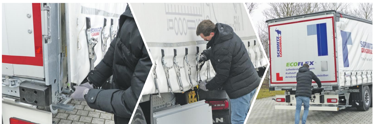
Routine: Ratcheting the tie rod into place tightens the tarpaulin horizontally. The tensioners are attached to the higher "short" position.
